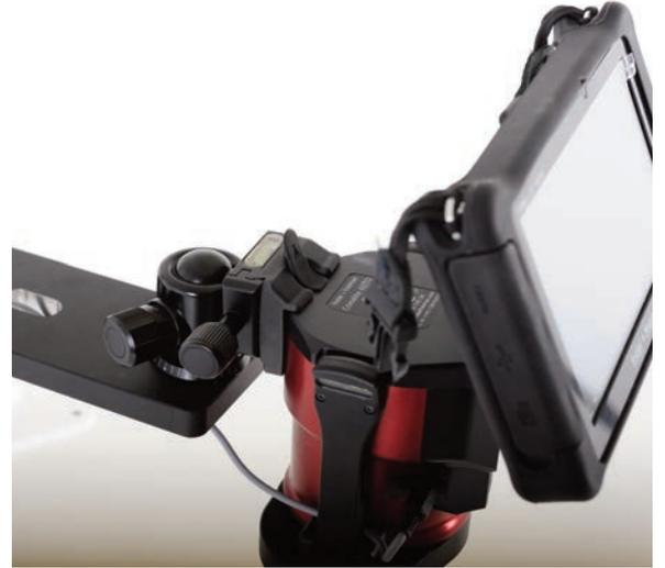
*The bench or wall mounted arm enables smooth operation of the Crime-lite AUTO in the laboratory*
